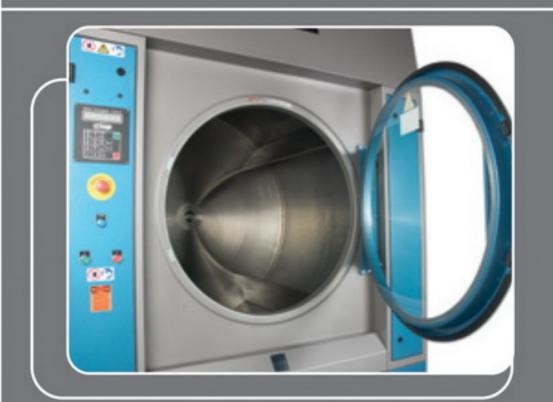
The large door opens 180 degrees making loading and unloading easy. The door glass is attached to the door without any gasket providing a long lasting door that offers security and low maintenance over the life of the machine. The door is provided with a safety switch that stops the machine when the door is open. A magnetic latch holds the door closed during operation. The door can be opened any time during operation for safety.
