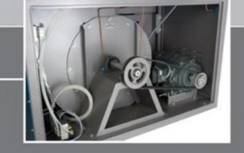
Totally enclosed motors are rugged and provide long life, meaning lint damaged motors are thing of the past. The machine is provided with a soft-start device for smooth starts and stops. A variable frequency inverter is available as an option.
