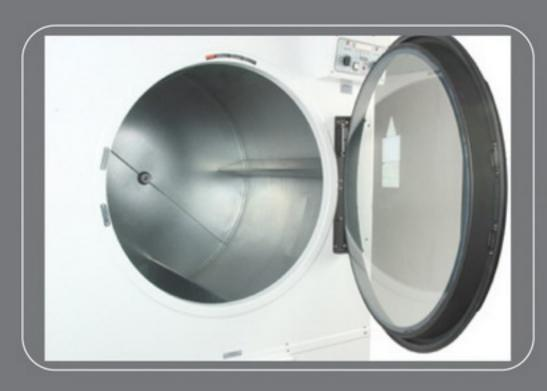
The large door opens 180 degrees making loading and unloading easy. The door glass is attached to the door without a gasket providing a long lasting door that offers security and low maintenance over the life of the machine. The door is provided with a safety switch that will stop the machine when the door is opened. A simple magnetic latch keeps the door closed during operation.
